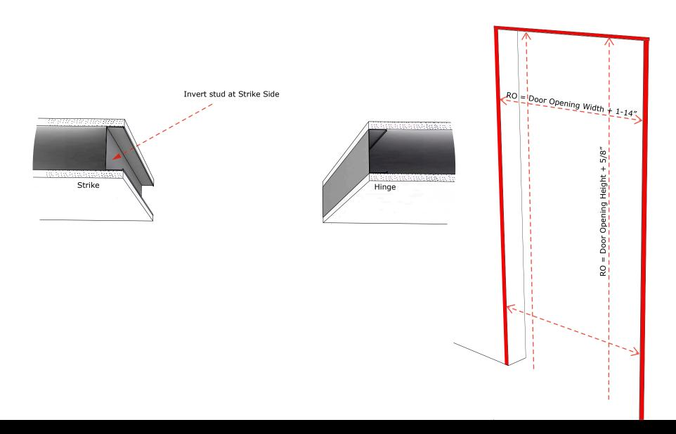
Slip header and vertical jambs into opening - Header will overlap jambs 3/8".
