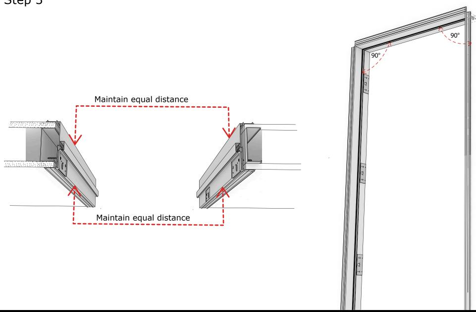
Attach four flat angles (C100ST) with #8 x 1-1/4" wafer head self drilling screws at all faces of jamb and header. Insure that screws pass through frame, gypsum board and into steel framing of partition.
