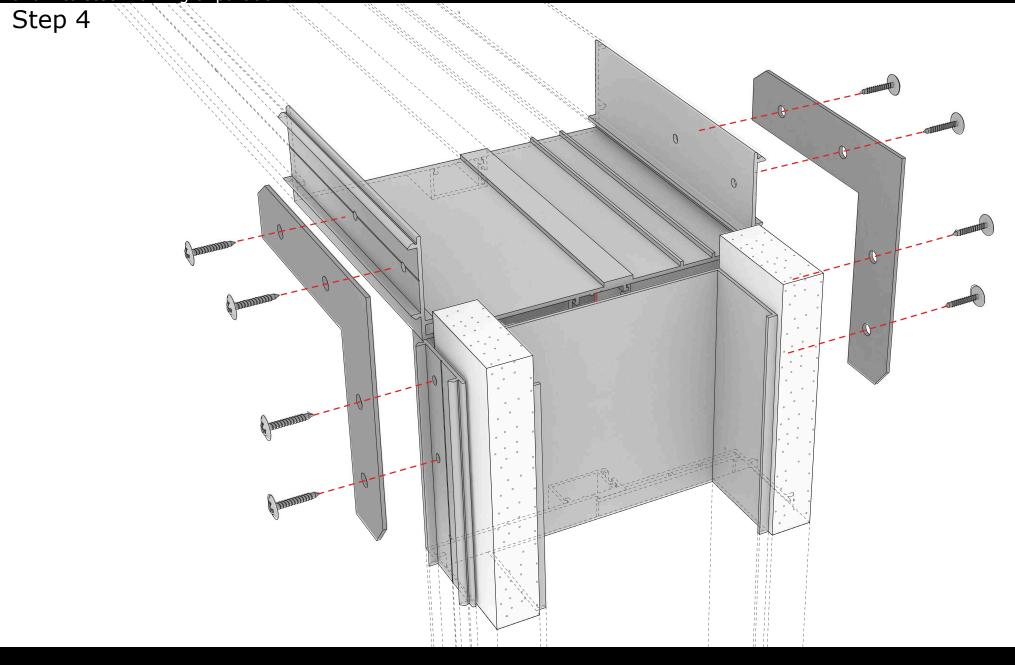
Check square, plumb and opening width. Anchor jambs to wall using  $\#6 \times 1-5/8$ " drywall screws through round holes nearest top and bottom of each hinge and 6" OC elsewhere. Attachment should roughly align on both front faces.
