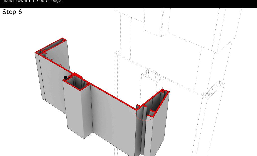
Anchor hinge plates to metal studs using the provided #10 x 2" screws.
