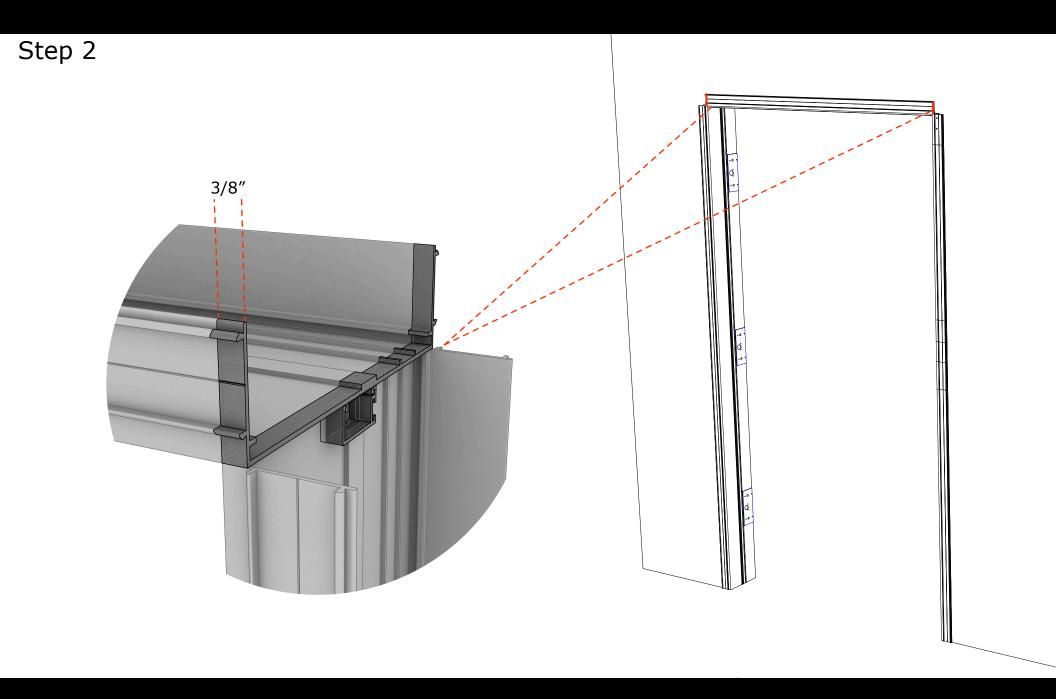
Align to scheduled opening width and height, achieveing equal wall capture on both jamb legs. Check level of header, square and plumb jamb legs.
