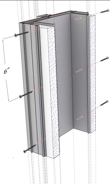
Install trim by hooking inside leg on the reciever tab and tapping lightly with a rubber mallet toward the outer edge.
