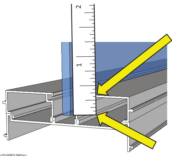
Minimum of 5/16" at the header and vertical jambs. Minimum of 1/8" at the base.
