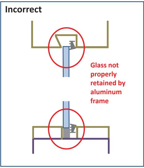
**Glass Bite dimension** (shown by the yellow star) is the distance that the glass sits inside the glass pocket of the glass jamb, or inside the glass base. A minimum of 5/16" bite is needed at the header and the vertical jambs, and 1/8" at the base.
