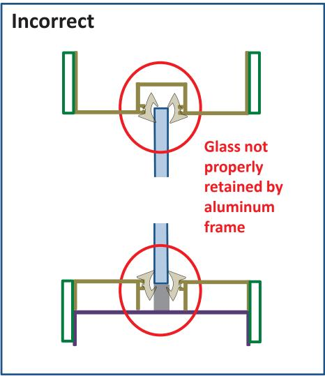
**Glass Bite dimension** (shown by the yellow star) is the distance that the glass sits inside the glass pocket of the glass jamb, or inside the glass base. **A minimum of 5/16" bite** is needed at the sides and header of the glass. At the base, a minimum of 1/8" is needed.
