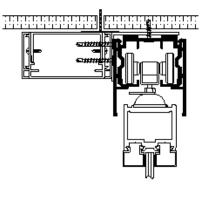
Hang Door by placing track in bottom rail on the door guide then push top of door to track and secure to rollers in track
