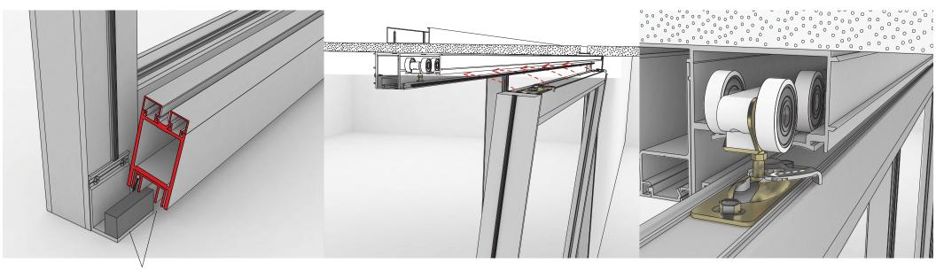
The door guide keeps the door sliding in the correct plane. The door may need adjusting up or down to ensure a smooth operation.
