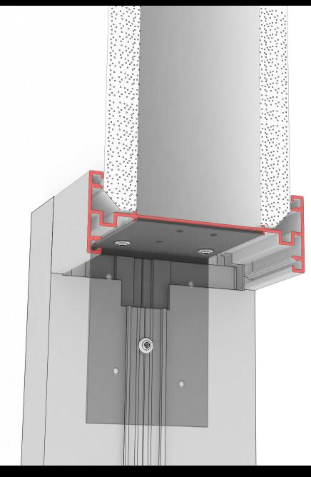
Slide the C400ST clip between the hinge jamb and hinge stud before putting the hinge jamb into position. Once hinge jamb is lined up correctly with H-Mullion header, attach clip to H-Mullion using two 1/2" tek screws. Then secure the hinge jamb to the clip with one 1/2" tek screw though the door stop retainer area.
