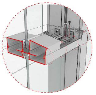
Attach the C406ST (mini clip) to both sides and each end of the horizontal glazing member using three 1/2" tek screws. The clips will mount on the bottom side of an H-Mullion, and the tops of glass base and mid-height base.
