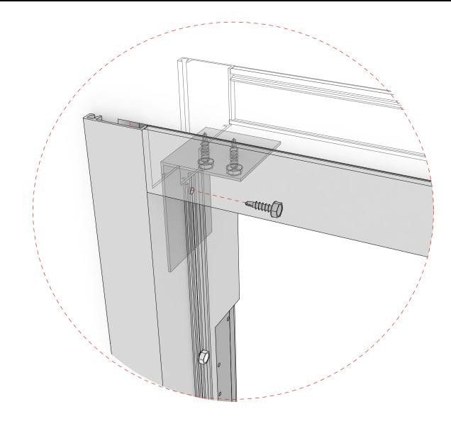
For freestanding single or pair Type 1 frames, the header clips are pre-attached at the factory to the header. Attach header to jamb with  $#10 \times 5/8$ " TEK screw in pre-drilled hole on jamb. Install screws at a slight upward angle to ensure a tight joint.
