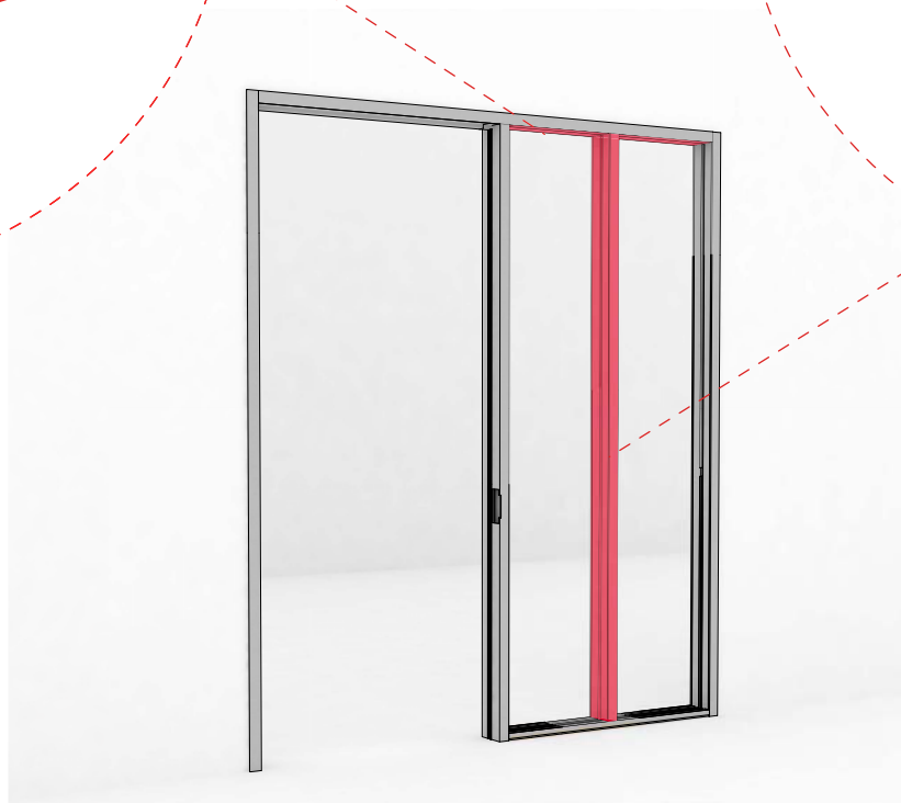
Snap glass pocket into vertical glass jamb.
