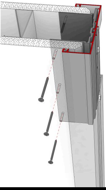
Attach vertical jambs to drywall partition with 1-5/8" drywall screws. Use a minimum of 3 screws per stud segment per side.
