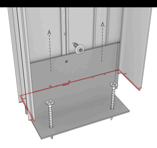
Slip the C210ST (floor clip) into the bottom of strike jamb behind extruded tabs and slide clip up so that the bottom of the clip and jamb align. Secure to jamb with 1/2" tek screw. Anchor the C210ST to the floor once in place. The method for anchoring is up to the installer.
