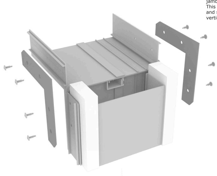
Use the C100ST clip to attach outside vertical jambs to a header with four 1/2" tek screws. This clip helps to ensure the opening is plumb and square. The header should sit on top of the vertical jamb and overlap the jamb by 3/8".
