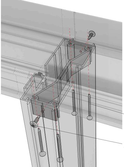
Locate the position of the BOSS clip and attach to the head condition using the provided  $#8 \times 1-5/8"$  flat head self drilling screws (4 required for each clip.)
