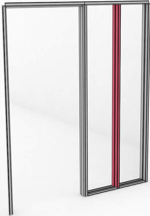
Insert glass pocket into glass jamb and secure with 1/2" tek screws at 18" on center
